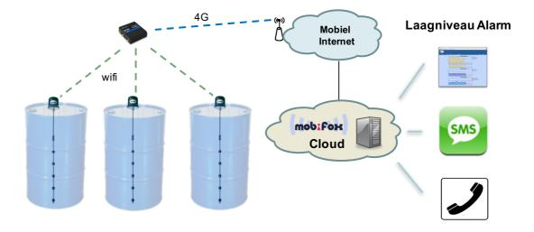
This unique MobiFlex level sensor can easily be mounted in the small (3/4 ") opening of a 200l or 60l oil drum. The MobiFlex is wirelessly connected to a central Mobifox Gateway. The Gateway collects all measured levels and sends it over 4G to the MobiFox Cloud. This Cloud server sends alarm messages when the level in the tank reaches a se alarm level. The sensor can be extended up to 3m.
